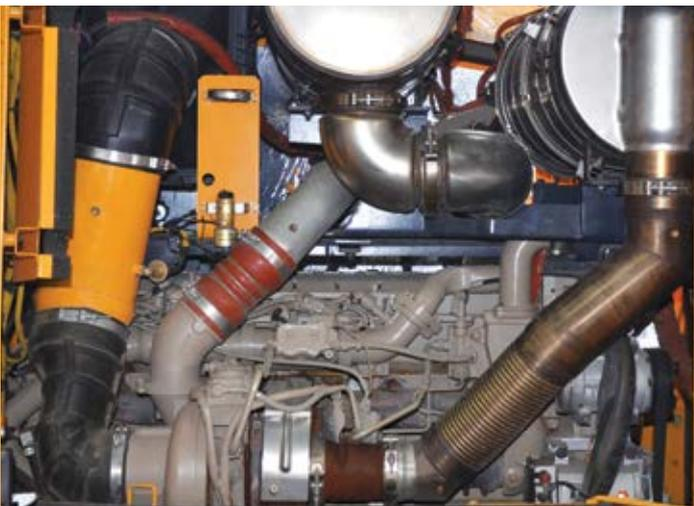
A dependable Cummins engine offers a high-pressure common-rail fuel system ensuring optimum, efficient performance while after-treatment technology including oxidation catalyst, diesel particulate filter, selective catalytic reducer, and AdBlue (DEF) injection and control system keeps the engine running clean.
