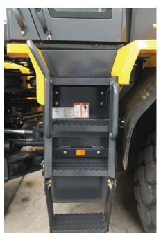
Access to the front of the cab by the operator or service person is a new feature. The same anti-slip bars used on the egress steps are used here for maximum anti-slip protection.
